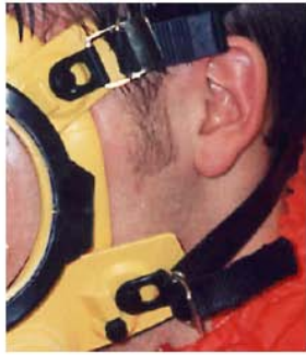
Figure 10 Loose head harness straps on a full face mask
